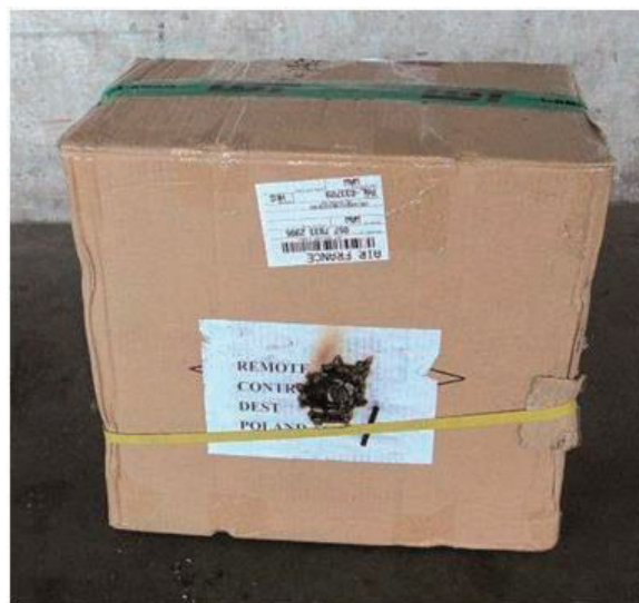
Figure 3. Fire damage to a package of incorrectly packed lithium metal button cells, which occurred after unloading
