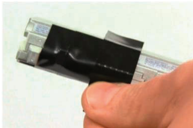
Figure 4.1. Protecting the exposed terminals of a spare laptop battery with insulation tape
